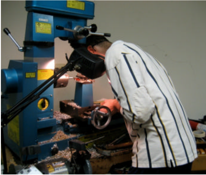
Fig1: First, turn down the outside of the bar stock to the desired diameter (approximately 1/2"). This dimension will be the diameter of the flange that holds the insert from the outside. Make the center hole a bit smaller than 6mm to allow for reaming later).
