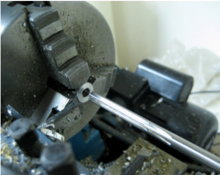
Fig5: Ream the hole to exactly 6 mm
