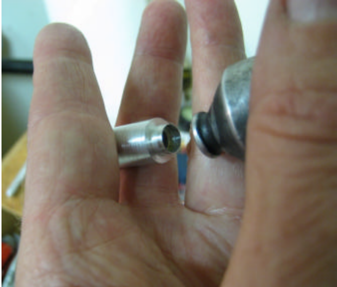
Fig3: Turn down the outside diameter for a snug fit into the end of the muffler. It's a good idea to measure an assortment of mufflers in advance. Although the rules state a maximum outlet diameter of 8 mm, many of the mufflers may be undersize. It's much easier to turn down the O.D. of the insert at this stage than once the part is finished.
