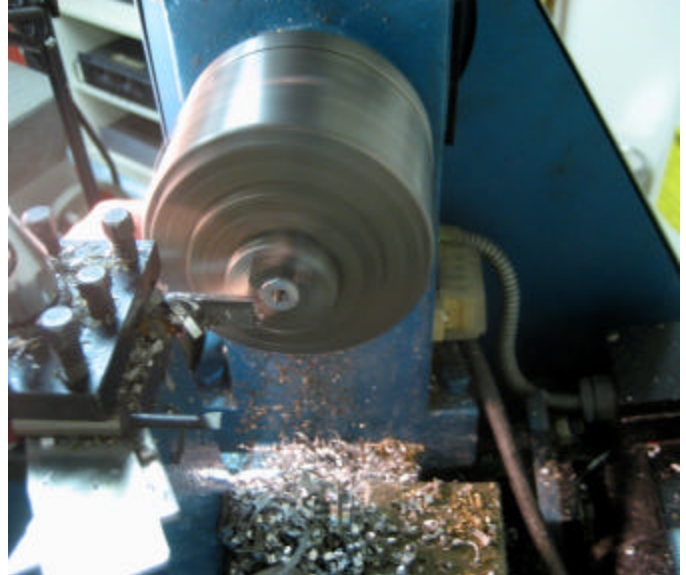
Fig4: Turn the part around and carefully re-chuck into the lathe. The wall thickness will be quite thin now (just the difference between the approximately 8 mm O.D. and the 9/32" internal hole). Cut off the part, leaving a 1/16"-3/32" flange with the smaller (6 mm) I.D. hole.
