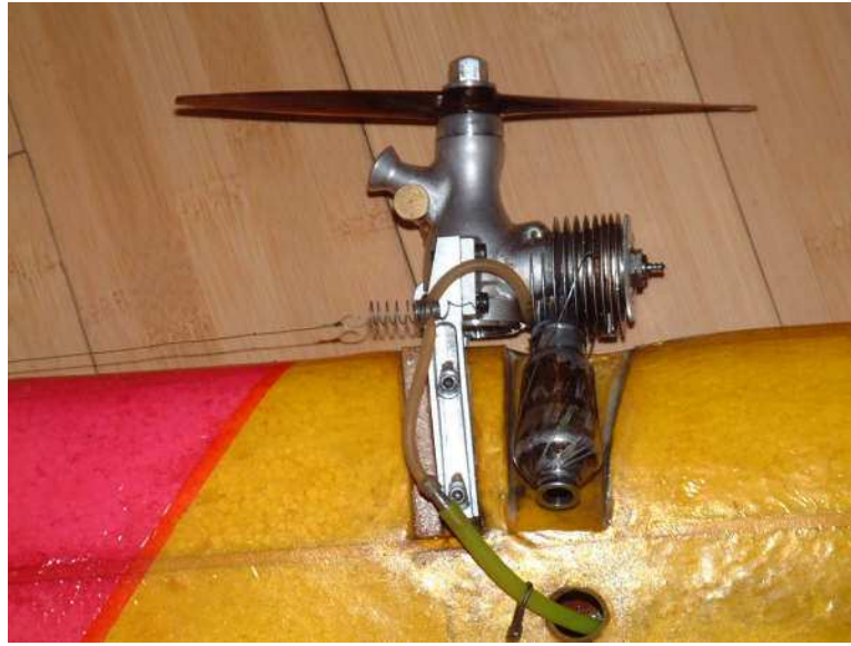
FIG. 1: Pete Athans' F2D shutoff. The other end of the string is attached to the leadouts, and opens the spring when line tension pulls the leadouts straight.
